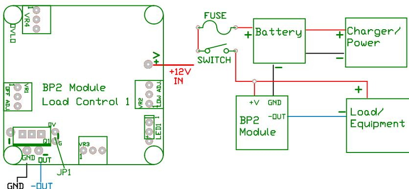
Load power control w/load shunt, EXT ON/OFF
