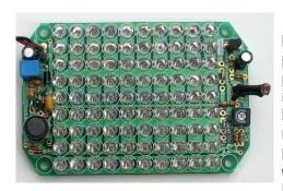
The LLIA90 is a high-quality and high-performance multi-purpose LED illuminator array. It has a built-in regulator and a photocell control circuit for automatic LED array on/off
