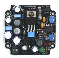
The SRD power converter is a high frequency, switch-mode, step-down regulator for applications requiring stable power. The compact and efficient design requires little heatsinking or support components. It provides the functions of bench-top power supplies in a
