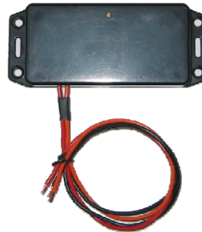
Battery Protector module inside plastic enclosure
