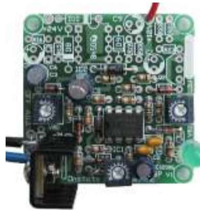
More function unit (CIR-BMBP-12V-2). Heatsink added for higher current (optional)
