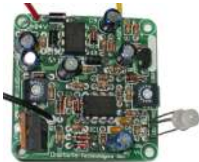
12V electronic fuse CIR-BMBPE-12V-1. 12V full function (-3) and relay version (-4) (power relay optional)
