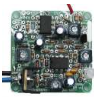
12V electronic fuse CIR-BMBPE-12V-1. 12V full function (-3) and relay version (-4) (power relay optional)
