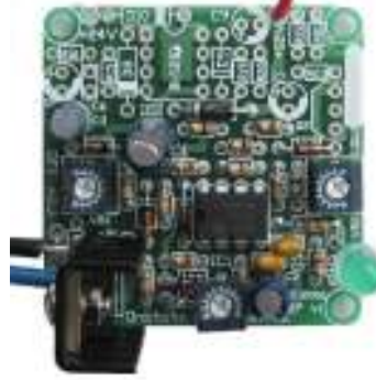
More function unit (CIR-BMBP-12V-2). Heatsink added for higher current (optional)
