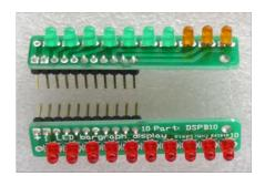
The DSP10 is a multi-purpose 10-LED bargraph display PCB for use as a stand-alone bargraph display or with Onstate bargraph meter modules. It is designed for use with 3mm LEDs and common positive wiring. A custom 10-segment LED display using multiple colour LEDs will provide a bright, appealing look to the project. Its small size, multi-function design makes it very useful as multi-purpose indicators not possible with standard 10-segment bargraph displays.
