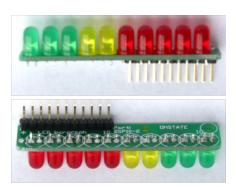
The DSP10 is a multi-purpose 10-LED bargraph display PCB for use as a stand-alone bargraph display or with Onstate bargraph meter modules (BM-4). It is designed for use with 3mm and 5mm LEDs with common positive wiring. A custom 10-segment LED display using multiple colour LEDs will provide a bright, appealing look to any project. Its small size, multi-function design makes it very useful as multi-purpose indicators not possible with standard 10-segment bargraph displays.
