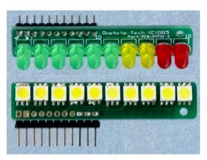
The DSP10 is a multi-purpose 10-LED bargraph display PCB for use as a stand-alone bargraph display or with Onstate bargraph meter modules(BM-series). It is designed for use with 3mm, 5mm, 5050 SMD or similar
