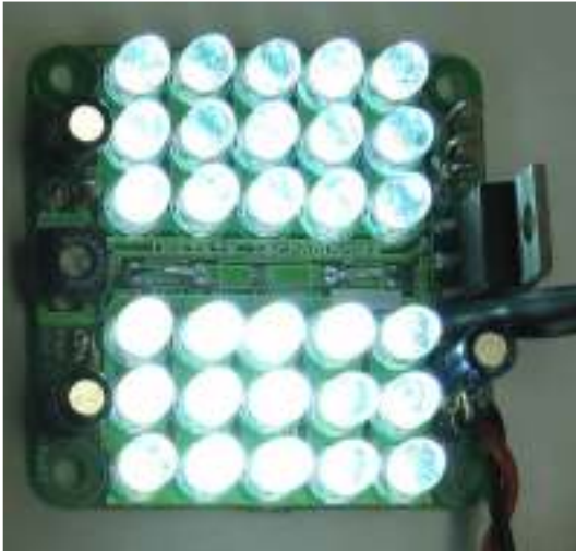
LLIA30 LED array. All LEDs operating.
