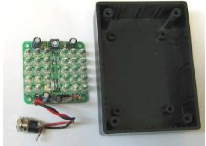
LLIA30 with parts. Drill holes on the side of the box to mount the 2.1mm jack.
