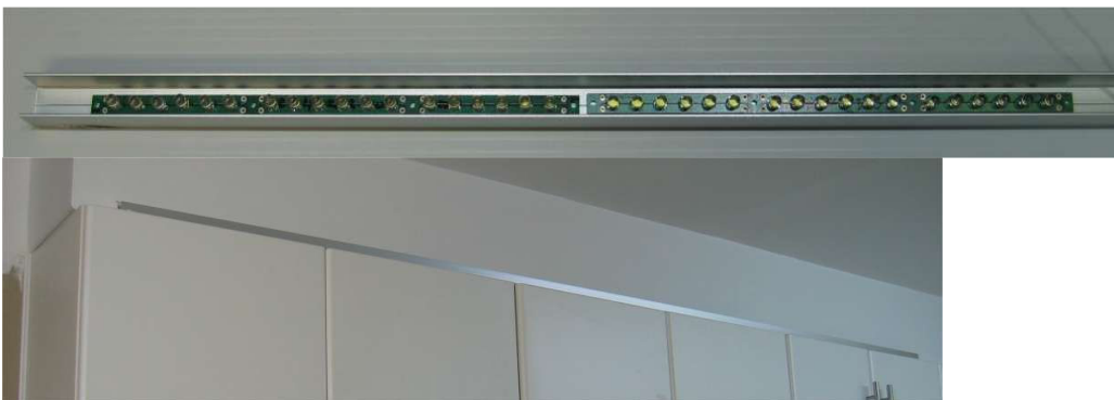
LED strip array inside aluminum U-channel for rigidity and covering.
