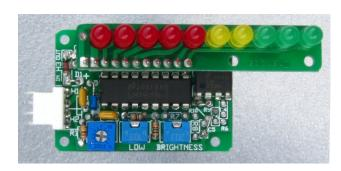
The BM Bargraph Meter is a 10-segment LED display meter for quick visual indication of voltage inputs or signal levels. Its small size, integrated, multi-function design makes it very useful as multipurpose indicators. It is compatible with the LM391x series of bargraph display drivers for linear or VU meter applications. The adjustable display scale range can be used for expanded scale voltmeters or signal displays.
