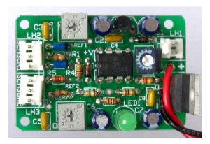
The PEMLT is an analog timer module for use with proximity, PIR motion and IR sensors to control LED lights. The circuit uses a dual op-amp for triggering and timing and an N-CH MOSFET for LED ON/OFF control. It is suitable for automatic lighting control in staircases, hallways, closets, cabinets, etc. The adjustable, multifunction, comparator-based design allows it to be used for other applications or for integration into other products.
