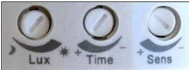
PIR motion sensor adjustment controls.
